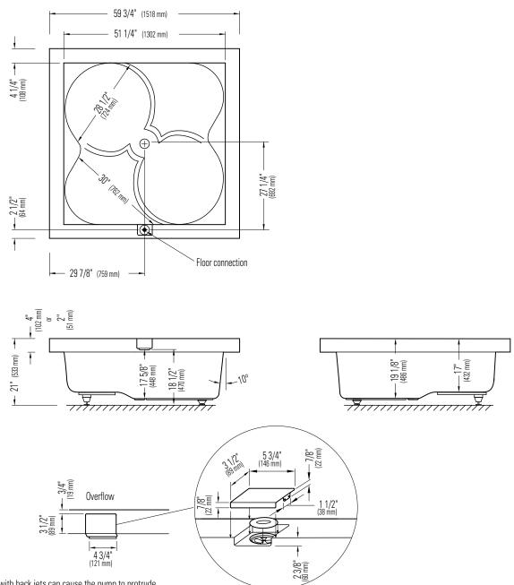
\*A bathtub fitted with back jets can cause the pump to protrude by approximately 3" from the overall dimension.
