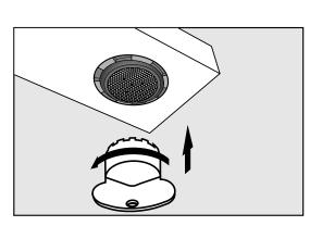
The nozzle position can be modified to change waterflow direction. To change it push the nozzle with your finger.
