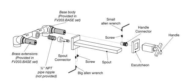
1- Make sure to place the valve with supply inlets pointed downward. The brass extension is already threaded onto the FV203.BASE body. It can be removed and trimmed using a saw along the provided groove, if necessary.
