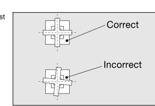
10 -Once the handle is on position, use the provided wrench to adjust the escutcheon. Make sure the escutcheon matchs paralelly with the handle.
