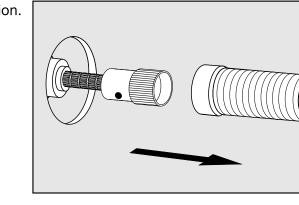
13- Remove, rotate, and reinstall the connector. And restart since point 6.
