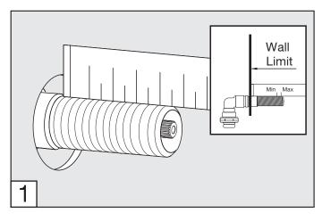
3 - <u>If the measured distance exceeds the</u> <u>"max" value</u> it's necessary to trim brass extension and valve stem (toghether).
